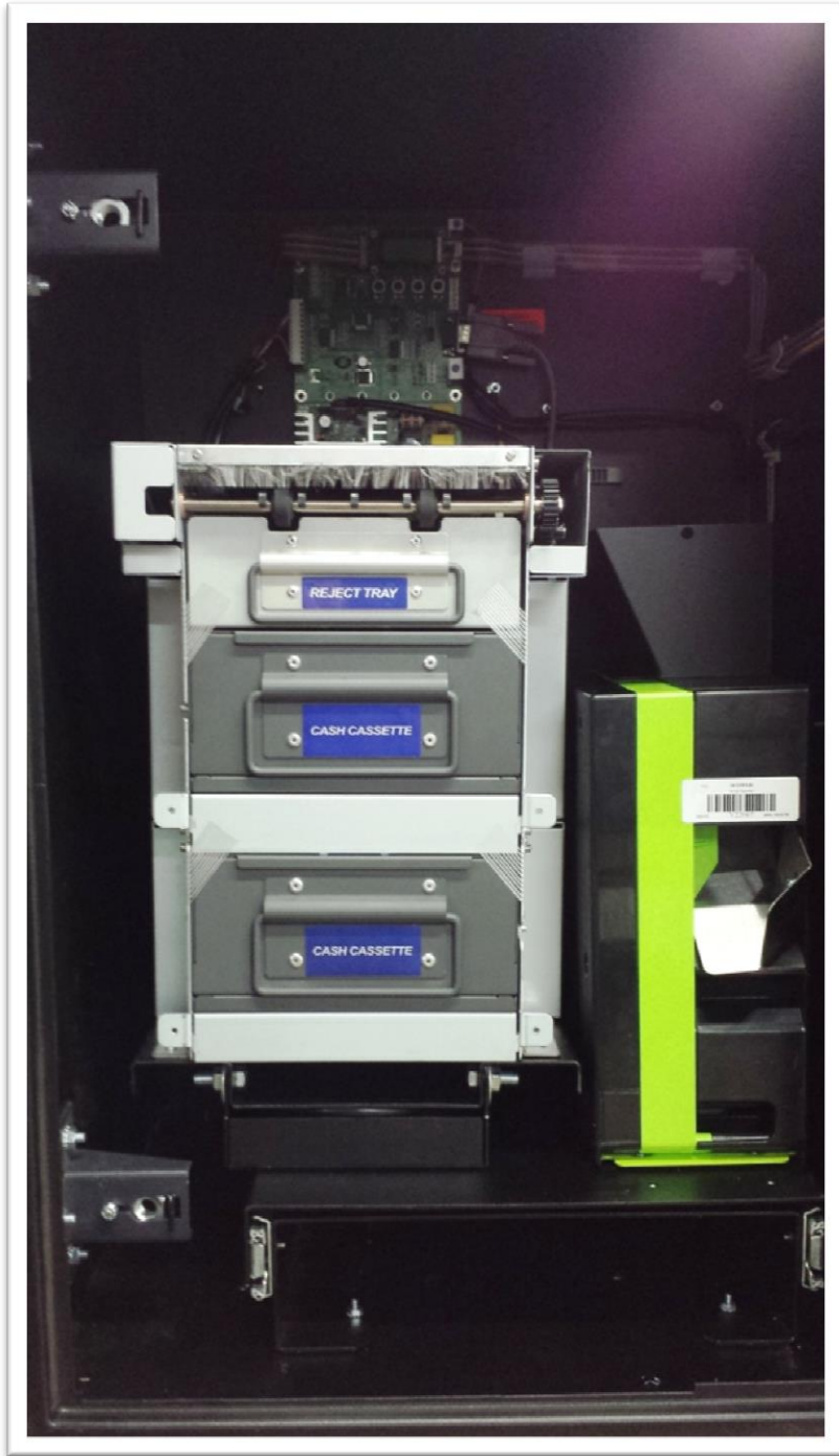
View of completed installation done on a front load model.
